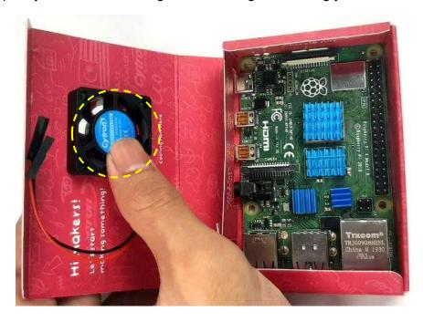
Align the cooling fan mounting holes with the 4 holes on the maker box. Insert **BLACK** rivets (from the top of the cover) and press firmly to secure the cooling fan in place.
