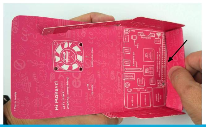
Fold the other right and left flaps inwards and slot the ends (marked "A") together as shown below.
