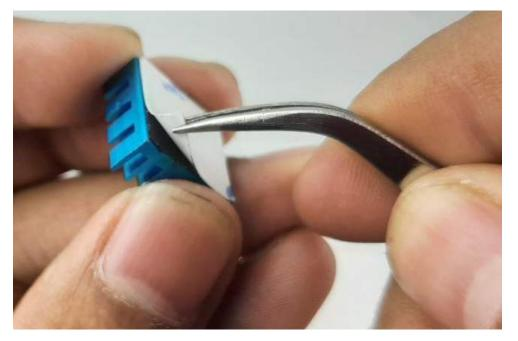
Attach all the heatsinks on the Raspberry Pi 4 Model B board accordingly.
