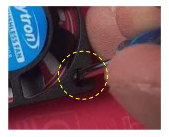
Push the center of the rivet until it loses its grip.
