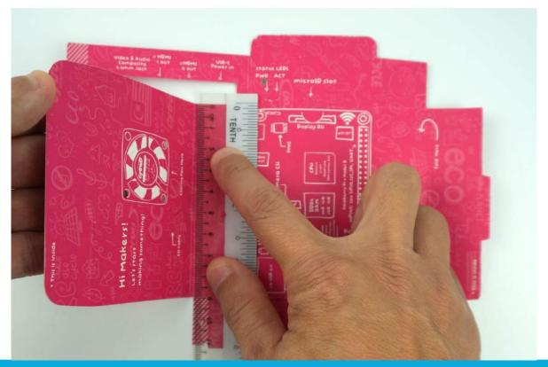
Fold up the side of the box that shows "microSD slot" and "Status LEDs" and the other side of the box that has openings for USB and Ethernet ports. And fold the right and left flaps inwards as shown in the image below.
