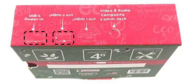
The box should look like the image below after the "USB-C Power in" and "µHDMI 0 out" openings are removed.
