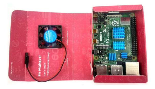
Place the Raspberry Pi 4 Model B board inside the box, hold and flip it over. We need to insert the rivets from the bottom of the box.
